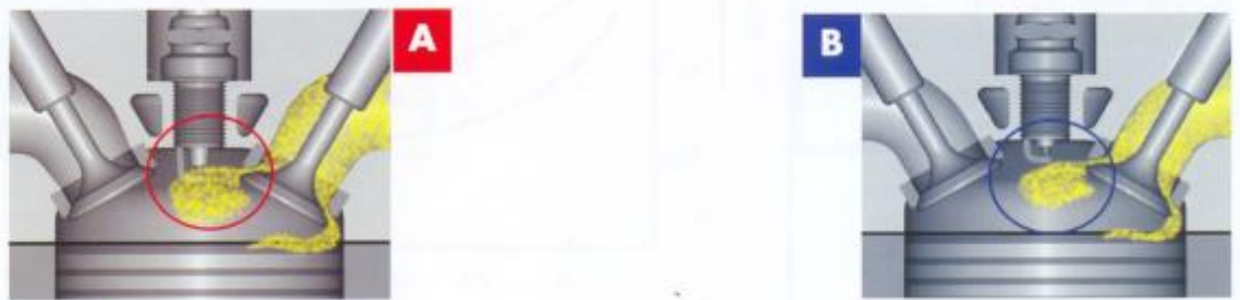
Influence caused by shifting the insulator tip out on thermal range extension
