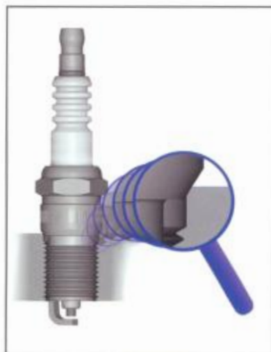
Methods of spark plugs sealing
