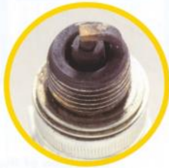
Fouling with dry combustion deposits
