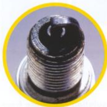
Fouling with non-evaporated fuel
