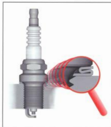
Methods of spark plugs sealing
